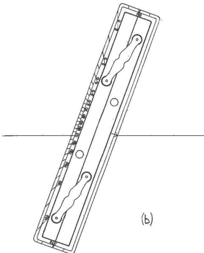
Fig. 4.2 (b) shows parallel rules matched on a parallel to an angle of  $70^{\circ}$ , thus indicating a direction on the chart of  $020^{\circ}$  T. or  $200^{\circ}$  T.
