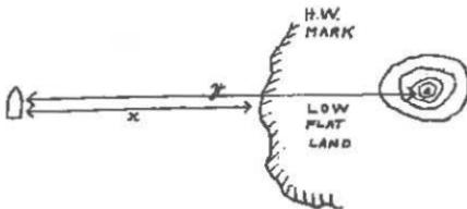
$x$  is the distance the vessel is actually offshore
