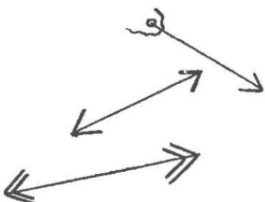
(a) A Terrestrial Position Line, i.e. a bearing from a shore object.
