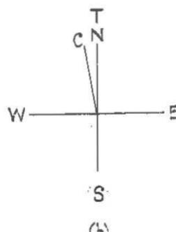
Vessel steering up the true meridian, compass error  $10^{\circ}$  E., gives diagrams as shown in fig. 10.4 (a) and (b).
