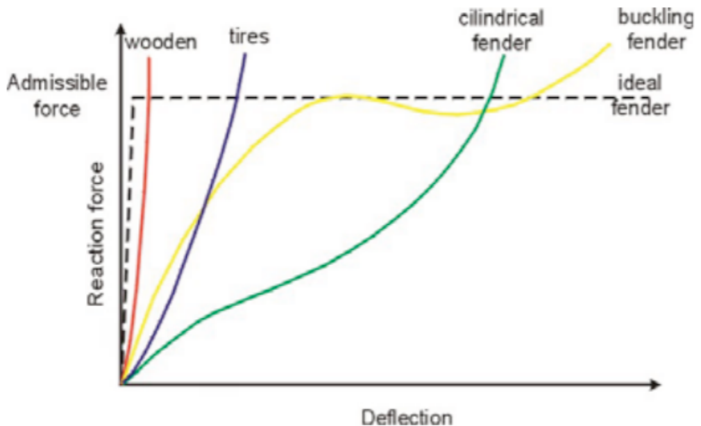
Figure 4 – Showing the deflection of different fender types
