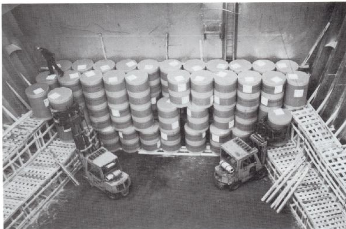
Newsprint loaded at forward end of hold. Note extensive bridging down the wings.
