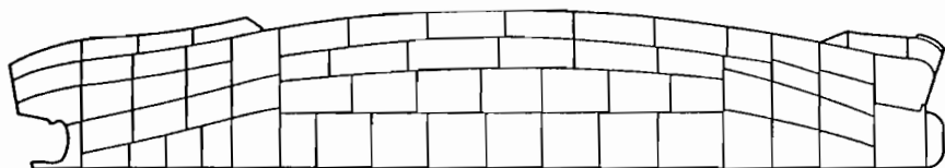
Figure 3.2 Shell expansion by units
