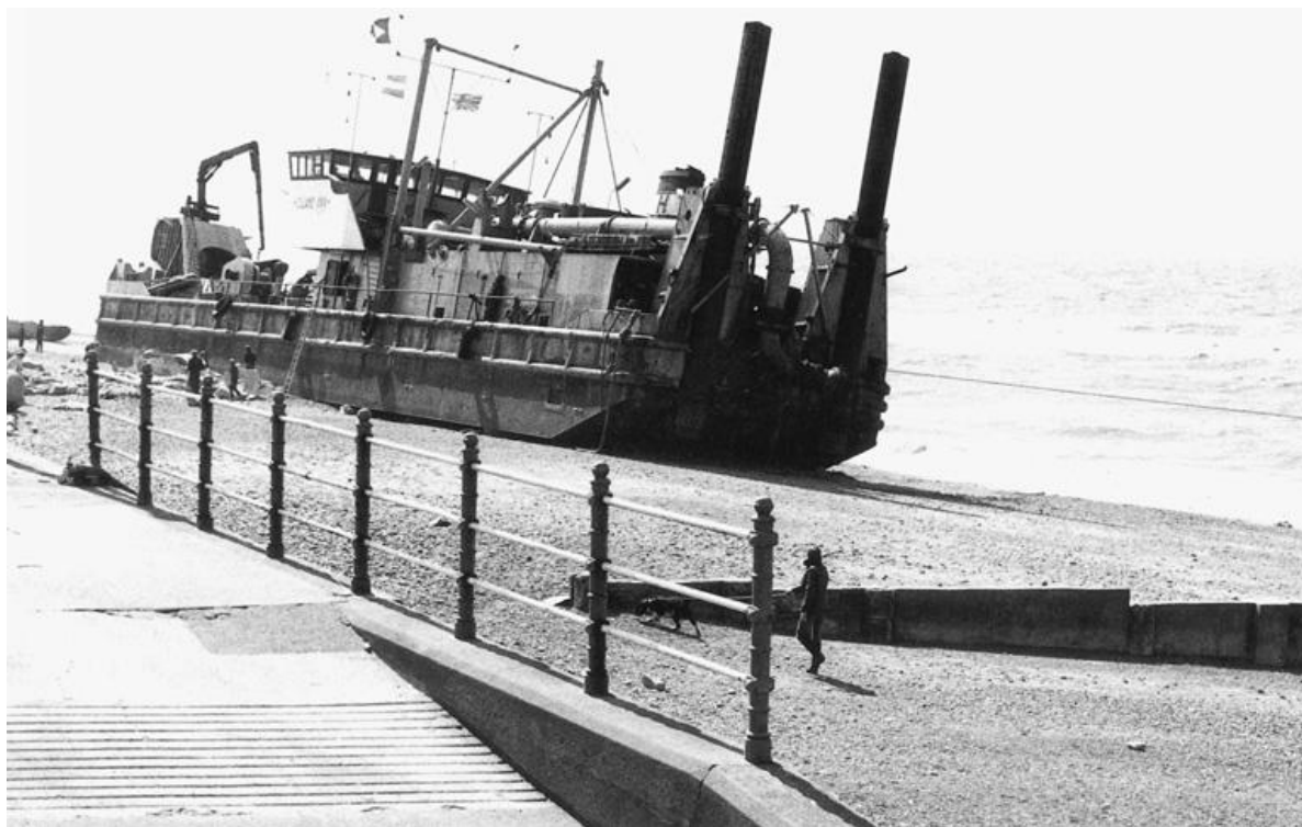
A flat bottomed dredger is blown ashore after losing her main engine power, onto a sloping sanding beach off a North West English coastline. Stay wires are seen, rigged to hold the vessel in position, to ensure she is not carried further inland on spring tides.
