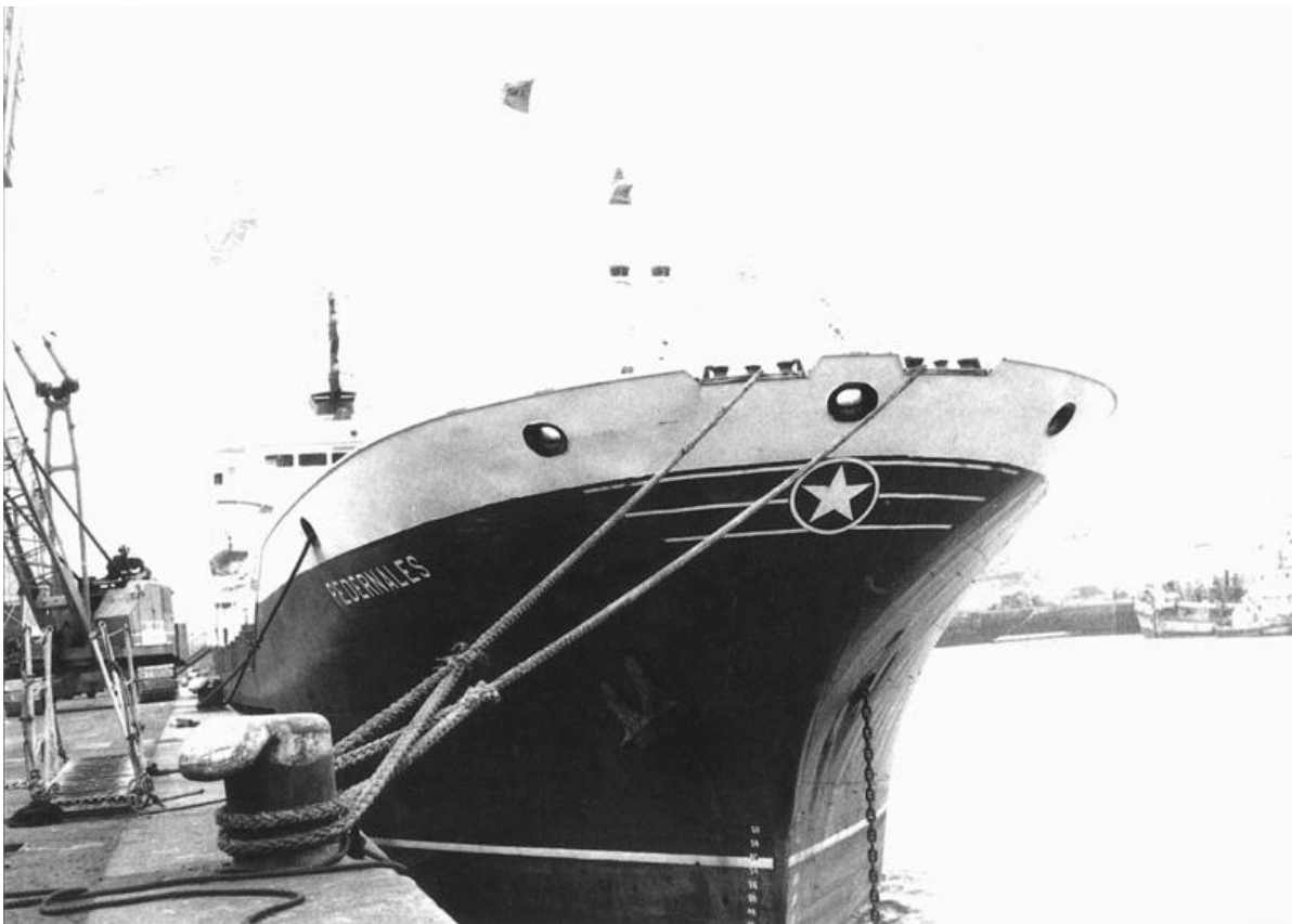
The vessel 'Pedernales' lies starboard side to, secured by two head lines and a rope spring at the forward end. The offshore anchor has been deployed during the berthing operation and the cable is seen walked back to an up and down position so as not to cause obstruction. Panama leads are seen centre on either side together with triple roller fairleads accommodating the lead for the head lines. Mooring ropes are soft eye, multi-plait polypropylene hawsers.
