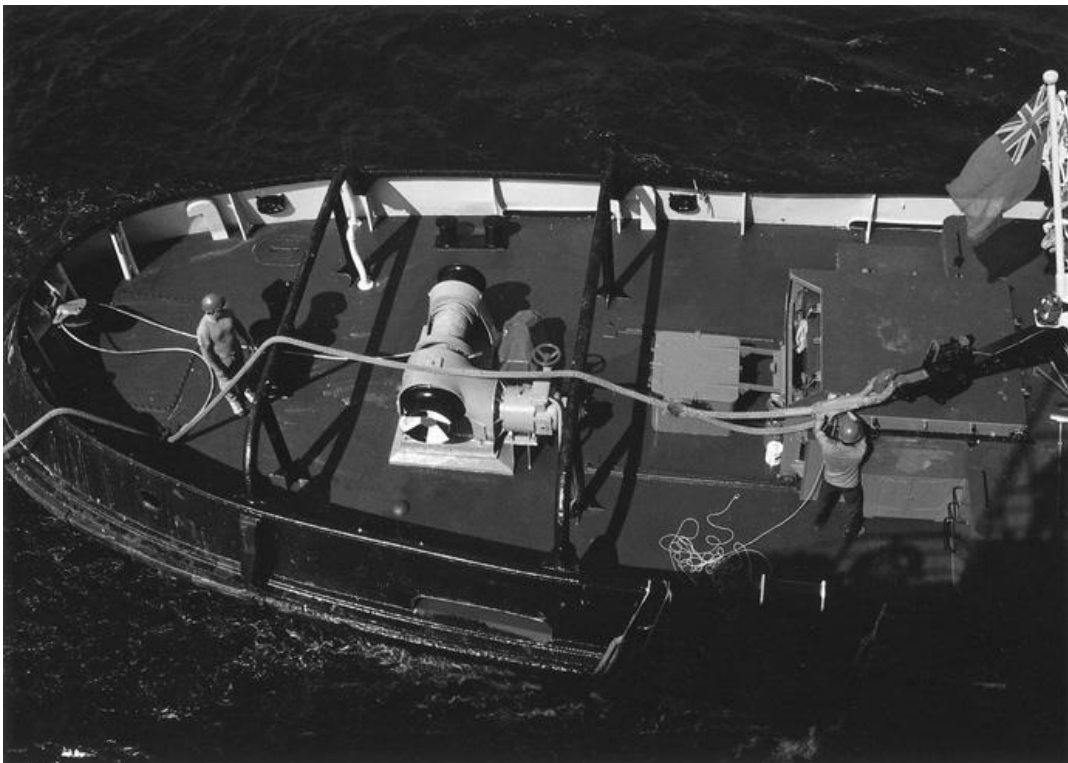
Tug Operations – securing the towline. The aft deck of an operational tug engaged in stretching a towline. The line is passed over the towing rails and secured by the 'soft eye' onto the amidships towing hook. A gob wire/rope arrangement is also set up in the slack condition, being led directly from the centre line winch through an aft lead, to a heavy duty shackle over the towline.
