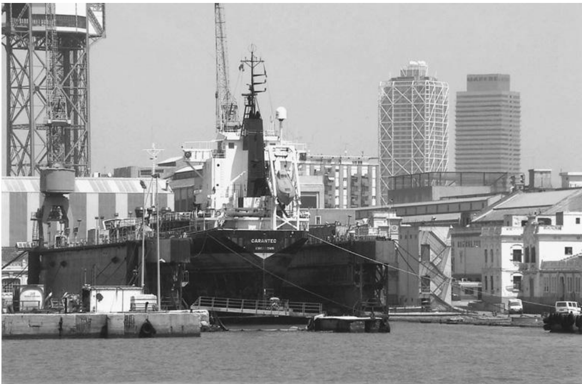
The 'Carantec' seen from the seaward aspect, lying in the floating dry dock. The floating dock is semi-permanently moored in the wet basin, allowing access from the inner harbour waters.
