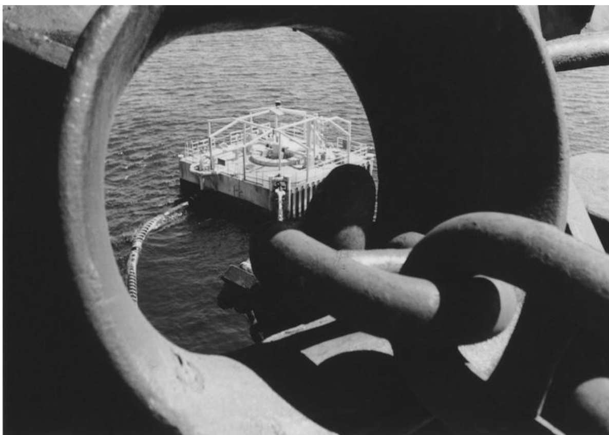
A chain mooring is sent away through a ship's lead to an SBM; once connected, the floating pipeline would be engaged to effect oil transfer.
