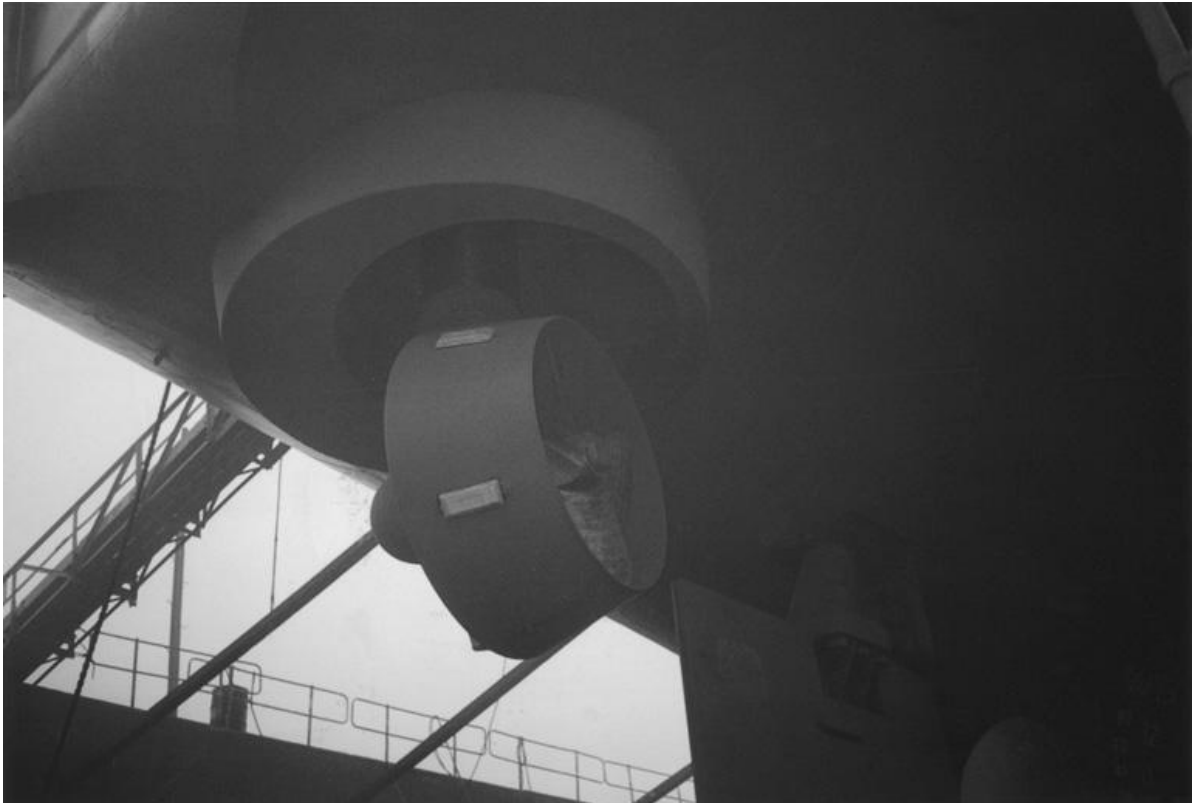
A ducted azimuth pod, featured on the outer hull port side, of a twin rudder/twin propeller vessel.
