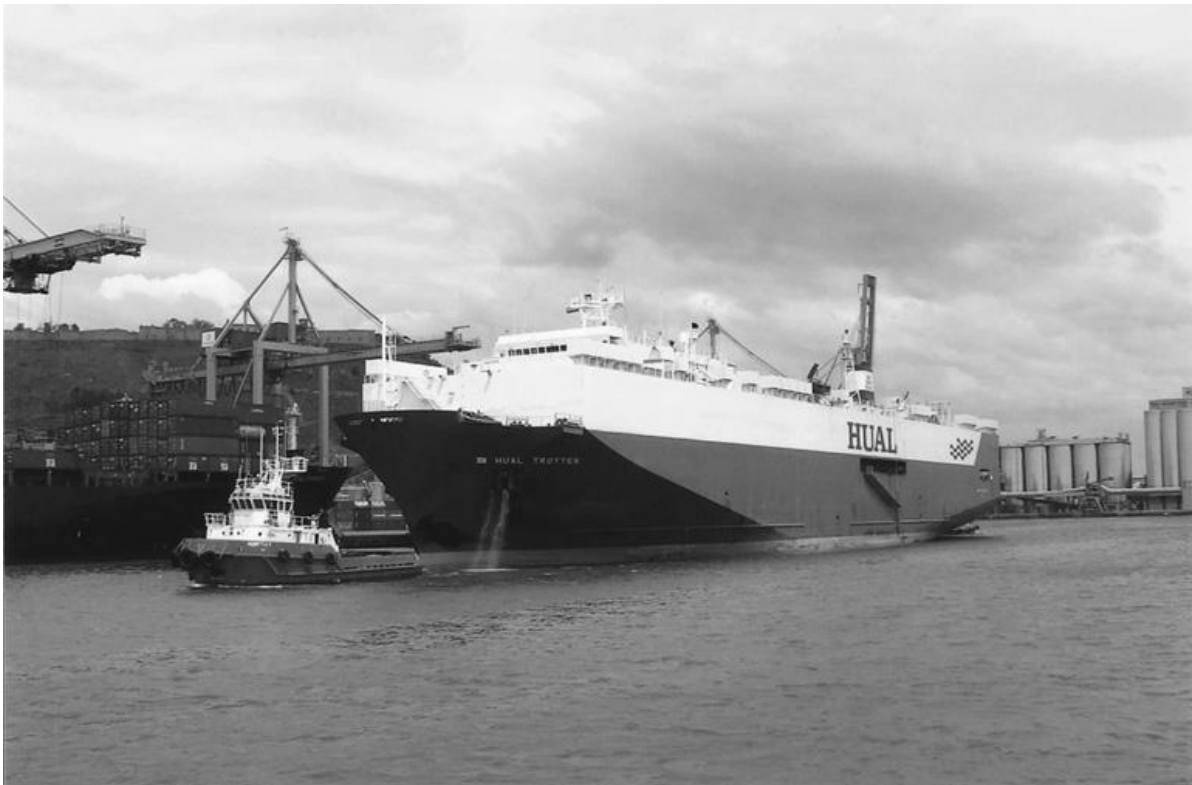
A small tug, seen engaged with the large carrier 'HUAL Trotter'. The danger of interaction is a one when small craft like tugs are engaged in close proximity to larger, parent vessels.
