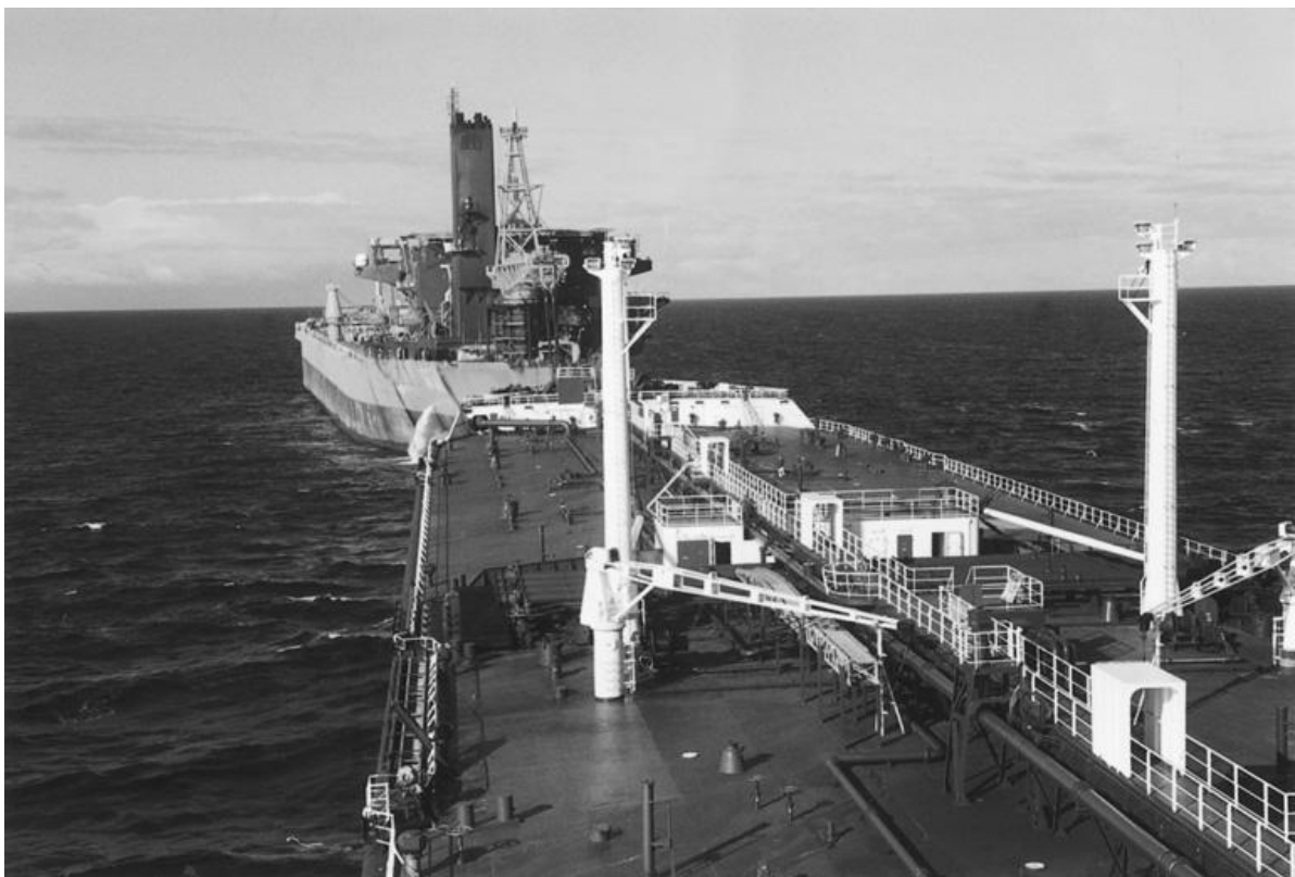
A large tanker manoeuvres in close proximity to an FPSO in offshore regions. Such close manoeuvres between vessels and fixed or floating structures are known to generate interactive forces which tend to hamper ship handling operations.
