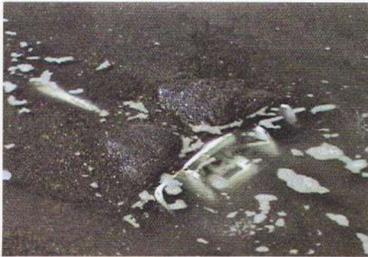
Fig.3-5 AC14 anchor biting into the bottom
